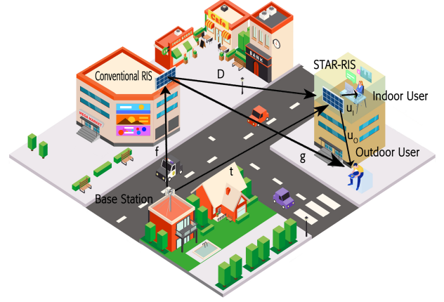
Fig. 1. Application scenario for double RIS-aided mobile communication.
