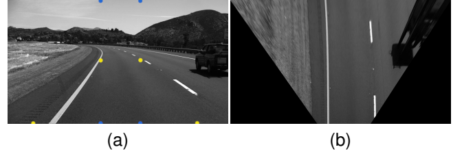
Fig. 3. A typical example of perspective change. (a) Marking the eight points used in the original image. (b) BEV image resulting from IPM.
