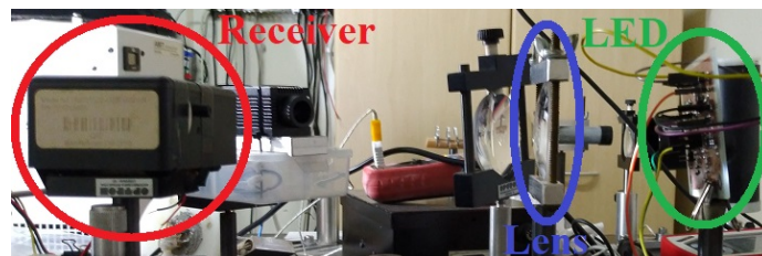
Figure 9. Experimental apparatus for optical power measurement. (Spectrometer is highlighted in red, the LED printed circuit board is highlighted in green, and an inert lens (without influencing the optical properties) to collimate the beam of electromagnetic radiation, between the light source and the receiver, is highlighted in blue).
