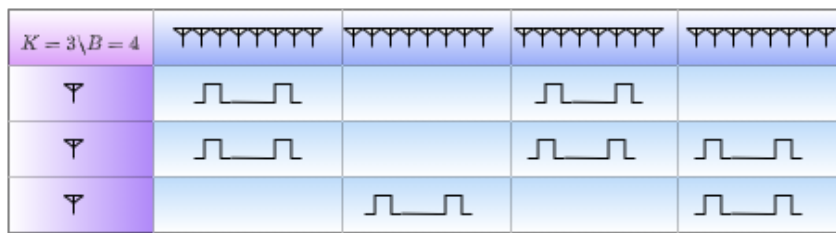
Figure B.2 – Arbitrary UL arrangement with P_a = 1 , K = 3 UEs (single antennas), M = 32 , B = 4 SAs ( M_b = 8 antennas) and \tau_p = 5 available pilot sequences. In this example, all UEs selected the same RA pilot.
