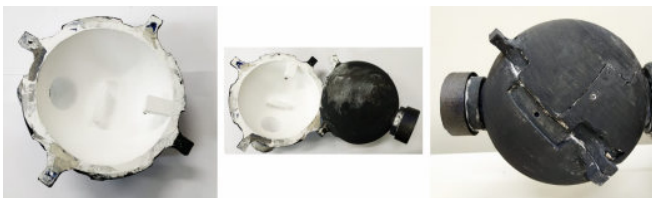
Fig. 4. Construction and painting of the smaller integrating sphere.
