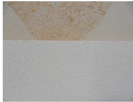
(b) Edge of a sheet of MDF in perfect condition after the cut.
