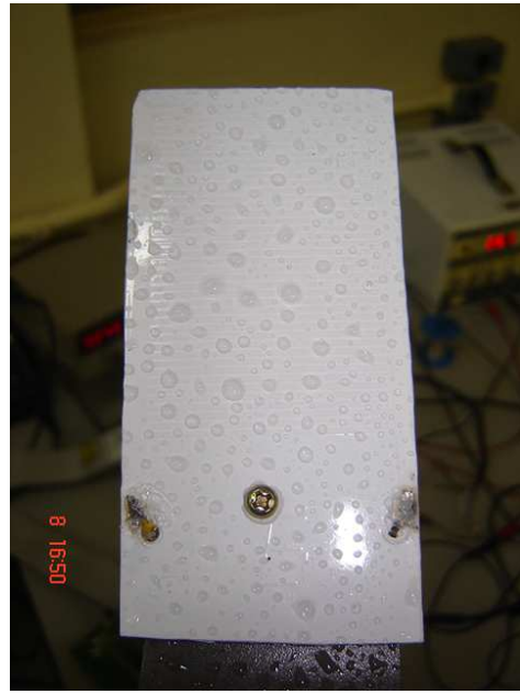
(b) Sensor coberto com tinta esmalte ( Cap\#(5, 6) );
