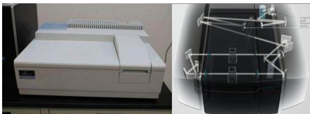
Figura 28 – Espectrofotômetro PerkinElmer UV/Vis Spectrometer Lambda 25 (RENZI, 2015).
